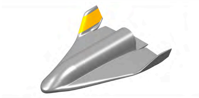
Figure 1: The SOAR shuttle highlighting the inboard winglet represented by a single NURBS patch. [Courtesy of S3, Swiss Space Systems Holding SA].
